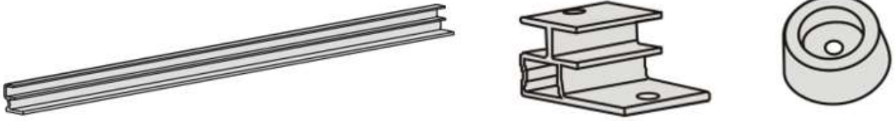
FIGURE 2—FROM LEFT TO RIGHT: AW-02 STARTER STRIP; AW-08 CLIP; T-07 EPDM SPACER
